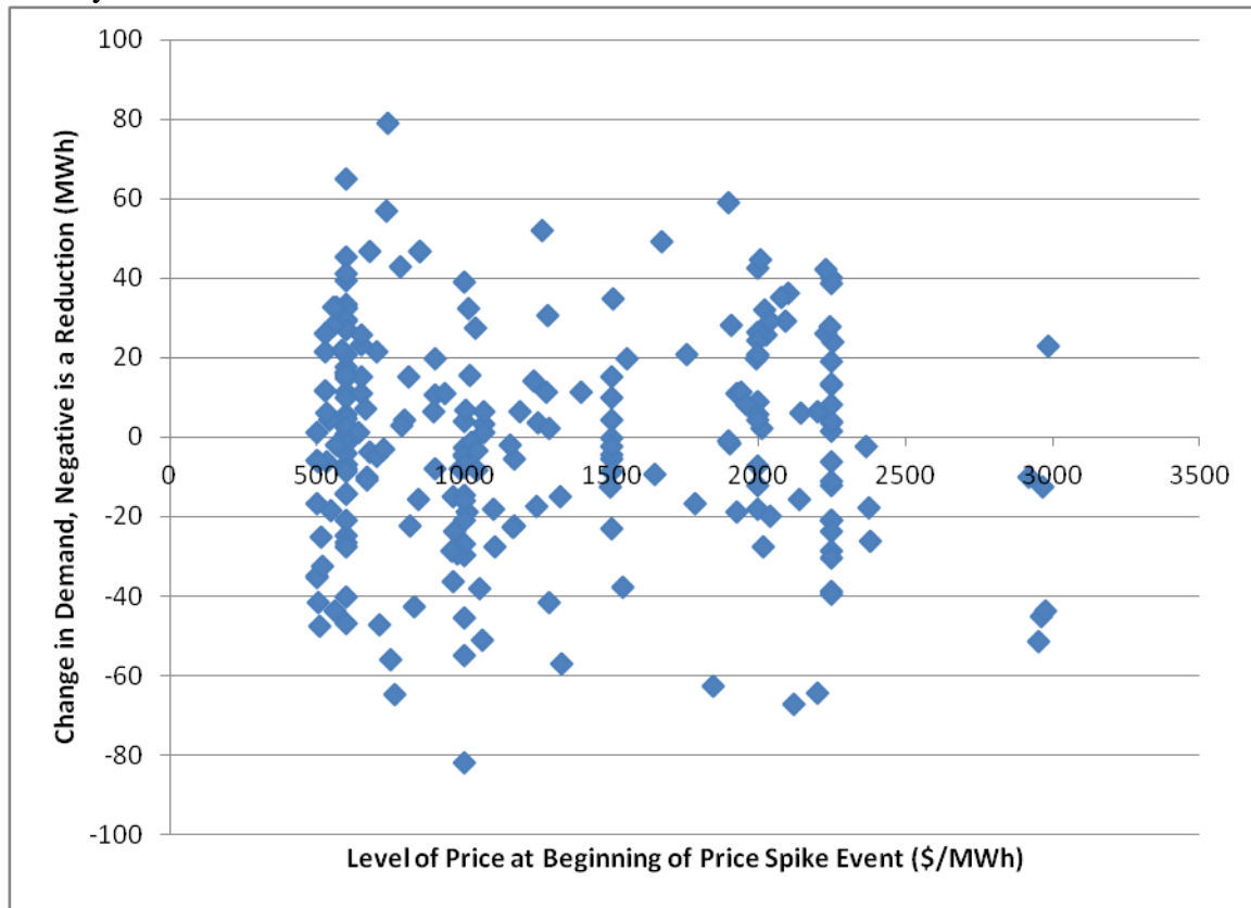
Figure 6 Average Reduction for Energy Consumers served at Transmission Voltage Based on Previous 5 Day Baseline or Same Interval as Previous Weekend Day if Weekend for all Price Spikes Since January 2007
